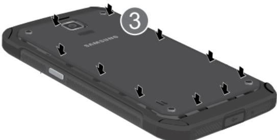
3. To avoid water damage, ensure that the back cover is completely closed by pressing in the centre until you hear a click.
