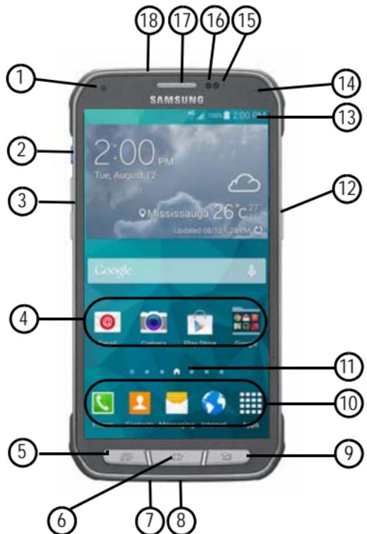
1. **Indicator light** illuminates with a series of distinct colors and flashing patterns to indicate different notifications and statuses. Events include Charging, Low battery, and Missed event:
