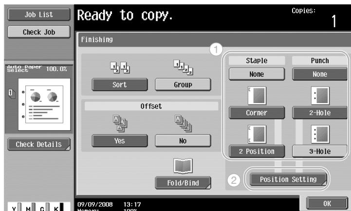
When select the Punch setting, specify the position where holes are to be punched.
